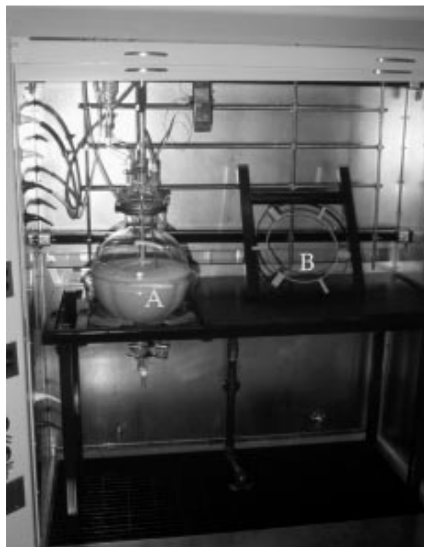
Figure 1. Photograph of a 22 L reactor vessel using the primary fume hood support (item A) and the primary fume hood support plus the adapter ring (item B shown without cushions). Note the easy access to the space under the reactor.
